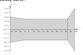
Analog error: max  $\pm 0.1\%$  FS, after calibrated at 25 °C Analog output thermal effect:  $\pm 0.007$  % FS/°C
